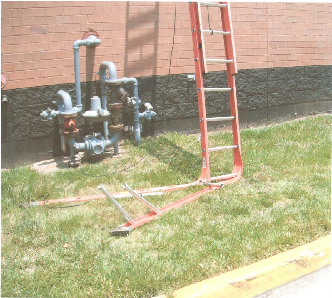
The lower section of the ladder failed
